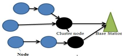
Fig. (1): PEGASIS basic structure protocol
