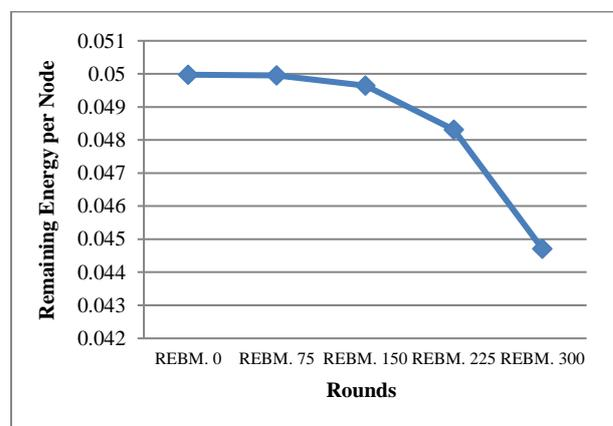
Fig. 4: Remaining energy per node (before movement)
