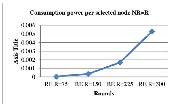
Fig. 5 d Consumption power radius (new radius=R)
