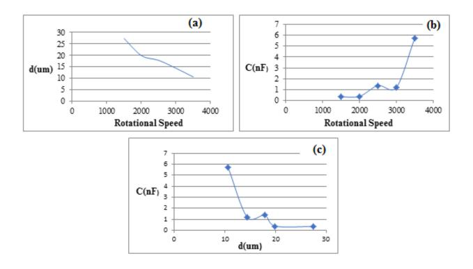
**Fig. (6)**: Thin film thickness for PMMA: a) film thickness versus Rotational speed, b) capacitance versus Rotational speed, c) capacitance versus thickness.
