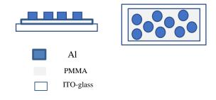
Fig. (2): The structure of capacitor (ITO/PMMA/Al).
