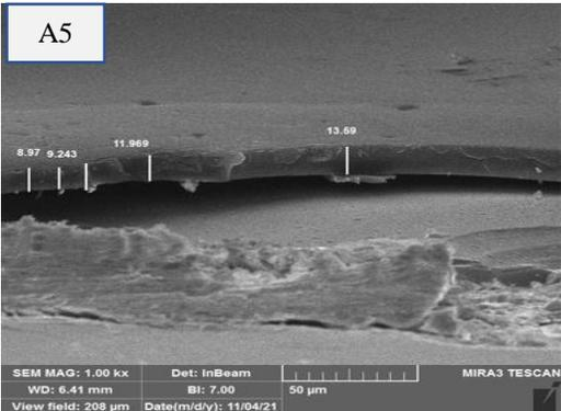
**Fig. (3):** FESEM cross-section for PMMA thin films A1(1500rpm), A2 (2000rpm), A3(2500rpm), A4 (3000rpm), and A5(3500rpm).
