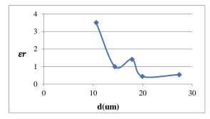
**Fig.(5**): The dielectric constant versus thickness for PMMA.
