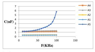
Fig.(4): the capacitance vs. frequency for polymer PMMA thin films.
