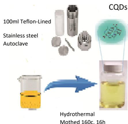
**Fig (1):** Synthesis of CQDS from PEG by Hydrothermal method.
