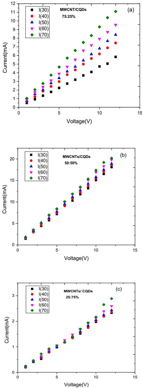
**Fig(6):** I-V Characterization for MWCNTs film Nanocomposite with CQDs.
