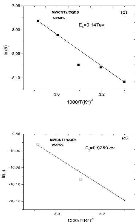
**Fig (8):** relationship between  $\ln(\sigma)$  and  $1000/T$  for MWCNTs film Nanocomposite with CQDs.(a).75:25%,(b)50:50%,(c)25:75%
