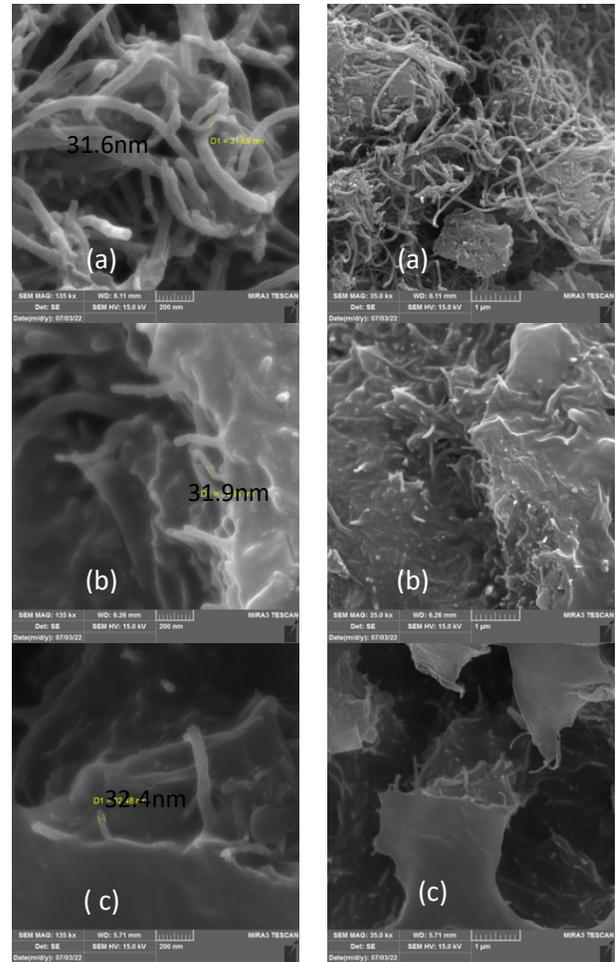
**Fig(4):** FESEM image of MWCNTs with Nanocomposite CQDs (a)75:25% (b). 50:50% (c) 25:75%.
